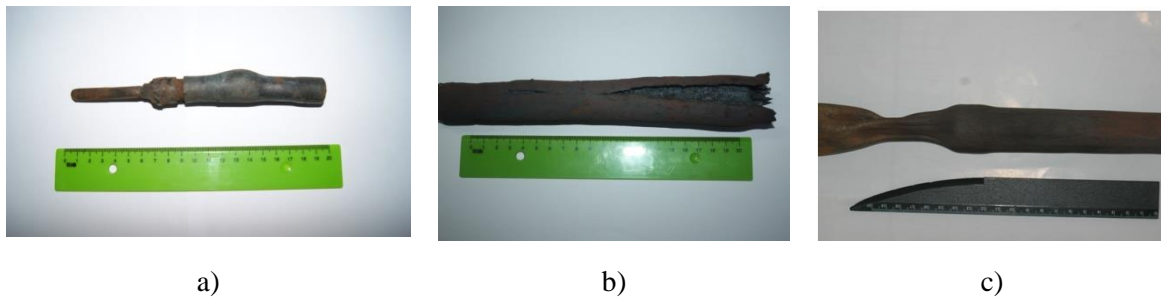
Figure 2 - The view of HEC billets based on Ta-Al precursors consolidated with intensity of loading under 10 GPa. a) Heating of predensified Ta-3Al billets above 950°C with further SHS reaction; b) HEC of Ta-3Al billet at 940°C, c) HEC of Ta-3Al-10% B4C billet at 940°C
