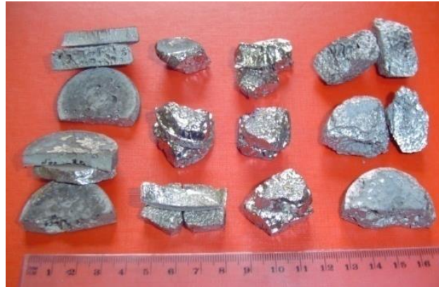
Fig 4 - Cast ligature with a different set of fusible and refractory elements
