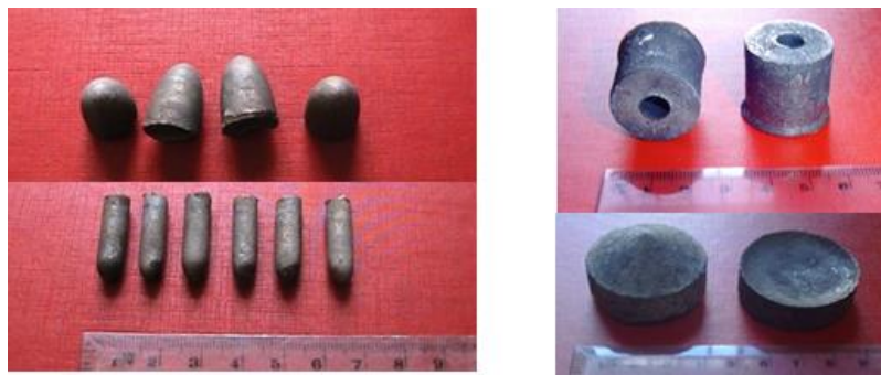
Fig. 2 - Examples of cast hard alloys materials with different configuration obtained under the influence of centrifugal
